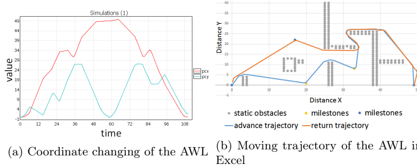
Figure 8.10: Moving trajectory of the AWL generated by the command {simulate 1[<=110] pcx,pcy} in UPPAAL SMC and exported in Excel
